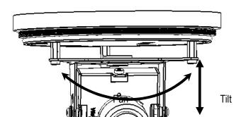
When you install on the ceiling, Change angle of view by turning this joint
